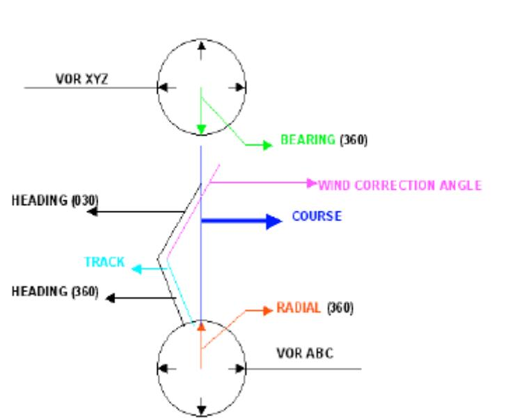
Let us consider the above diagram: bearing in mind that a VOR has 360 different Radials or if you want 360 compass degrees, where 360 degrees (note that 000 does not exist) indicates North, 90 degrees East, 180 degrees South and 270 degrees West.
