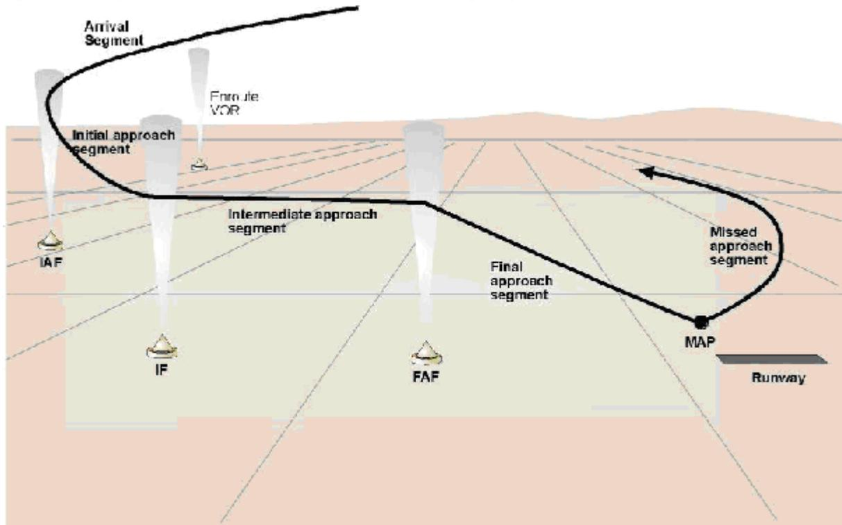
ATC may replace some or all (with the exception of the **FAF**) of these phases of the approach with radar vectors to the final approach, to allow traffic levels to be increased over those of which a fully procedural approach is capable. It is very common for ATC to vector aircraft to the final approach aid, e.g. the ILS, which is then used for the final approach. If traffic allows it or indeed if it becomes necessary then ATC can issue specific constraints on the approaching traffic:
