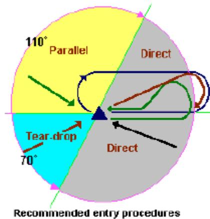
When crossing the fix to enter a holding pattern, the appropriate ATC unit shall be advised. ATC may also request that the pilot report “established in the hold”. The pilot is to report “established” when crossing the fix after having completed the entry procedure.
