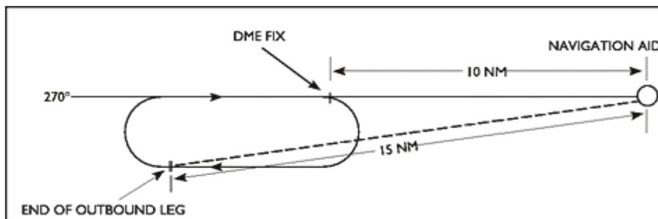
For example: An aircraft cleared to the 270° RADIAL 10 mile DME FIX, to HOLD BETWEEN 10 AND 15 miles, will hold inbound on the 270° radial, commence turn to the outbound leg when the DME indicates 10 NM and commence turn to inbound leg when the DME indicates 15 NM.
