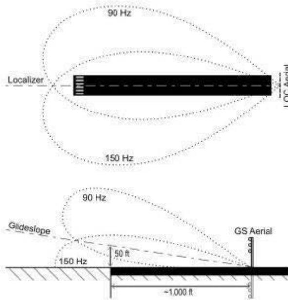
Normally approaching aircraft will be flying at an altitude which places them at an altitude between 3000 feet and 4000 feet to pick up the glide-slope. At times it is possible that due to temporary restrictions an aircraft may be coming in higher than normal in these cases the approach clearance needs to include the advise to the pilot that he can follow the glide or not to follow the glide as the case may be.
