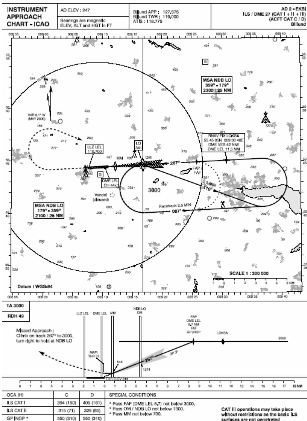
As you can imagine we do not want an aircraft circling at 3000ft over LO for too long, especially if there is more traffic inbound the field. So, prior to the aircraft arriving at LO, you could instruct the aircraft to leave LO on heading 110 for a left hand procedural approach back to runway 27.
