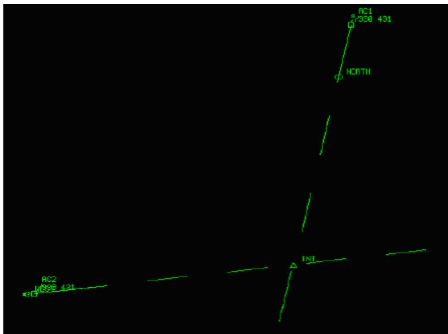
This is a typical situation: Two aircraft (AC1 and AC2) are flying on two different but intersecting airways using the same flight level. As a controller you have to consider all flights crossing an intersection point at the same flight level as a possible separation conflict. If you do not do anything then after about 3 to 5 minutes there two aircraft will be converging at the same altitude. Hence ATC needs to take action. If either of the aircraft is flying at a FL which is incorrect
