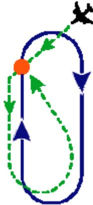
In a teardrop (or offset) entry, the aircraft flies to the holding fix, turns into the protected area, flies for one minute, and then turns back inbound, proceeds to the fix and continues from there
